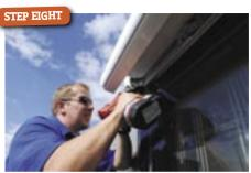
The final step to the fitment is to secure the awning in place using six small self-tapping screws. These don't take any weight - that's the job of the three large brackets - and allow the awning to be removed for either maintenance or cleaning.
