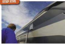
The wiring lead had to be extended in this case and this was carried out using crimped connectors. Next the hole for the 12V electric cable was drilled and the cable fed through to the interior.
