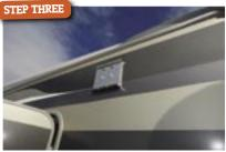
Once satisfied with the position, pilot holes were drilled and their position on the inside carefully checked. The holes were then enlarged to take the main support bolts. The plate itself can be attached with either silicone sealant (making it removable) or Sikaflex (which makes it stronger but permanently bonds the brackets to the body). Silicone was used here and can be seen oozing out of the lower holes.
